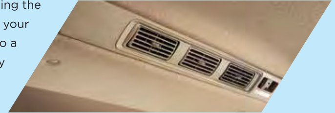
2nd Row Roof AC Vent
