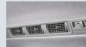
2ND ROW ROOF AC VENT
